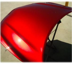
Clean Vivid Ruby is a tinted clear layer using specialised pigment dispersion technology to give the enhanced depth and clarity required in the latest OEM Candy Apple type colours. e.g. Ford Ruby Red.
