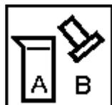
The topcoat and hardener should be thoroughly mixed before the addition of the SPP2000. Add 6% by weight of SPP2000 and thoroughly mix to ensure a completely homogeneous mix.
