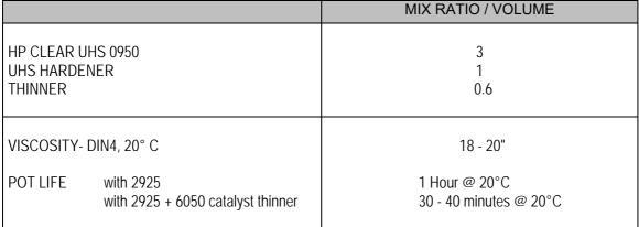
As with all Ultra High Solid products, cold ready for use paint temperatures can lead to more difficult application and overspray absorption. It is strongly recommended that ready for use product is applied at a temperature greater than 15°C.
