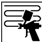
Number of coats: Apply 1 full single coat or 1 double coat to give a film thickness of 25-35 microns (1.0 - 1.4 thou.)
