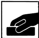
OE or existing paintwork should be sanded back to sound substrate layers using P320-360 grit discs (dry) or P600-800 grade paper (wet).
