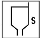
Spray Viscosity 16-18 seconds DIN4 @ 20°C
