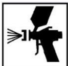
Spraygun set-up: 1.2 -1.3mm
