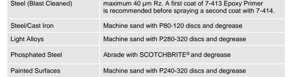
Blast clean to ISO 8527-1 SA 2.5 with a blast profile of
