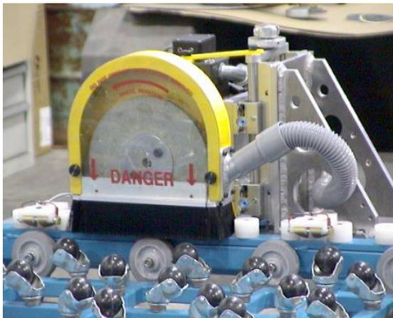
**Photo of Deletion Wheel and Dust Collection Enclosure on a Table Deleter.**
